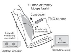
Fig. 1. Experimental setup used to evoke and measure the biceps brachii (BB) isometric twitch contraction responses. The TMG sensor measures muscle radial displacement during twitch contractions induced by short electrical stimuli. The stimulating electrodes are placed directly onto the skin.
