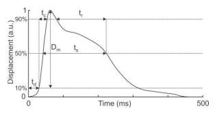
Fig. 2. (a) The parameters that were measured with the TMG signal: Dm - maximum amplitude (displacement), td – initial delay time, tc – contraction time, ts – sustained contraction time and tr – half relaxation time.
