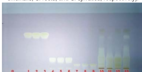
Figure 3. HPTLC chromatogram of polyphenols from Stachydis herba 20% methanolic extracts: white light illumination, derivatization with DPPH. B: Blank; Lanes 1–3: Caffeic acid, R_f 0.76; Lanes 4–6: Chlorogenic acid, R_f 0.22; Lanes 7–9: Rutin, R_f 0.08; Lanes 10–13: Samples ( S. germanica , S. officinalis , S. recta , and S. sylvatica , respectively).
