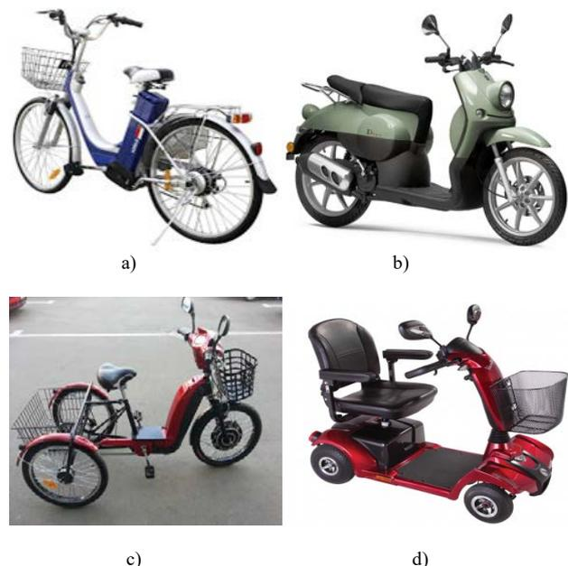
Fig. 1. Electrically driven light vehicles for people transport: a) bicycle; b) motor scooter c) tricycle d) trolley for disabled people.
