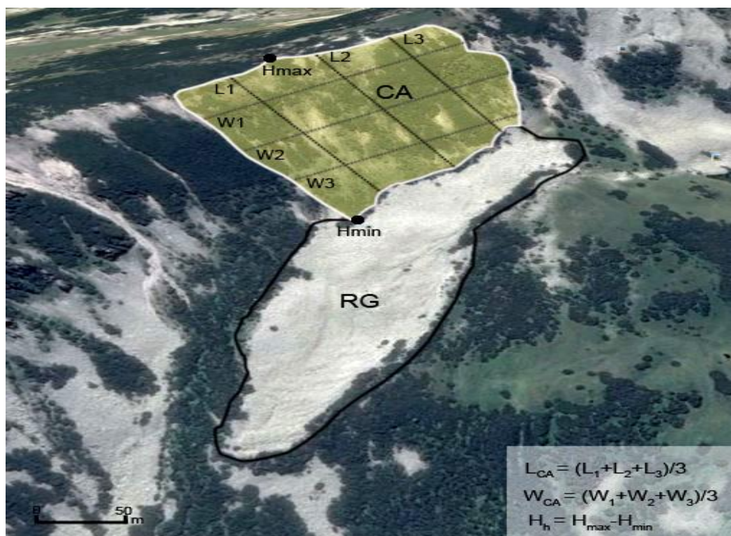
Fig. 2: Example of measurements for contributing area parameters (L - length; W - width; H – altitude)
