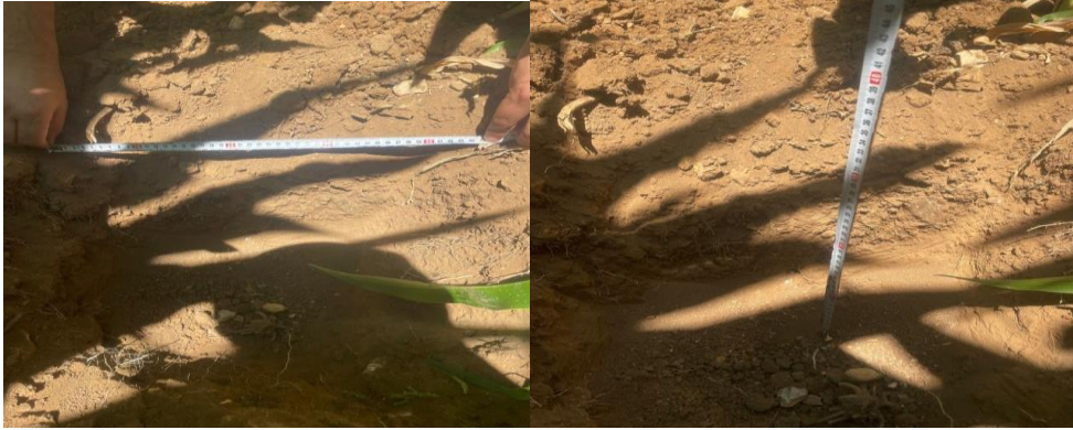
Figure 3. Water movement in soil profile under single drip lateral design for two plant rows
