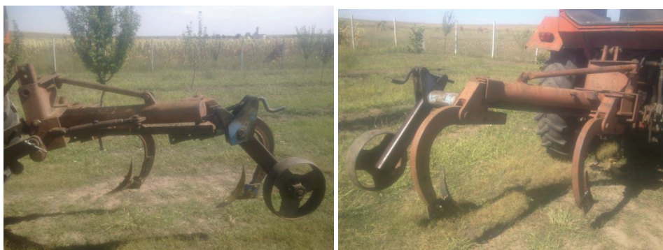
Fig.1. P 2VA plow equipped with raising organs.
